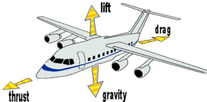
If these four forces are balanced, the plane will fly at a steady height (**altitude**) and speed (**velocity**). However, if one force is greater than the others it will affect the plane's motion through the air.
