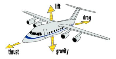
If these four forces are balanced, the plane with fly at a steady height (*altitude*) and speed (*velocity*). However, if one force is greater than the others it will affect the plane's motion through the air. *If...*
